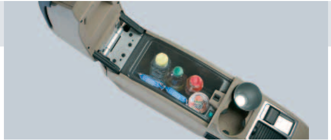
In der Premium-Konsole eingebaute Kühlbox In the premium central console integrated cooler box
